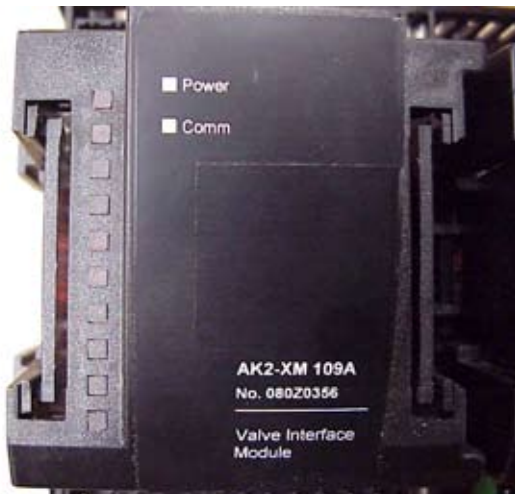
FIG. 54 - POWER AND COMMS LED'S
