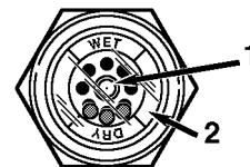
Receiver Tank Sight Glass
