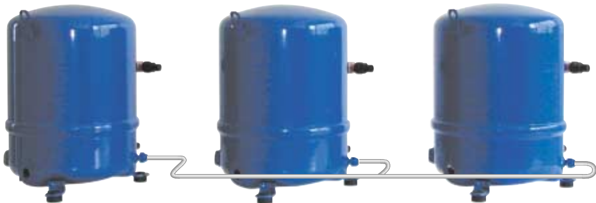
Figure 2.1 Example of correctly mounted oil equalization line system. Note all compressors are of equal size/capacity and mounted on the same level.
