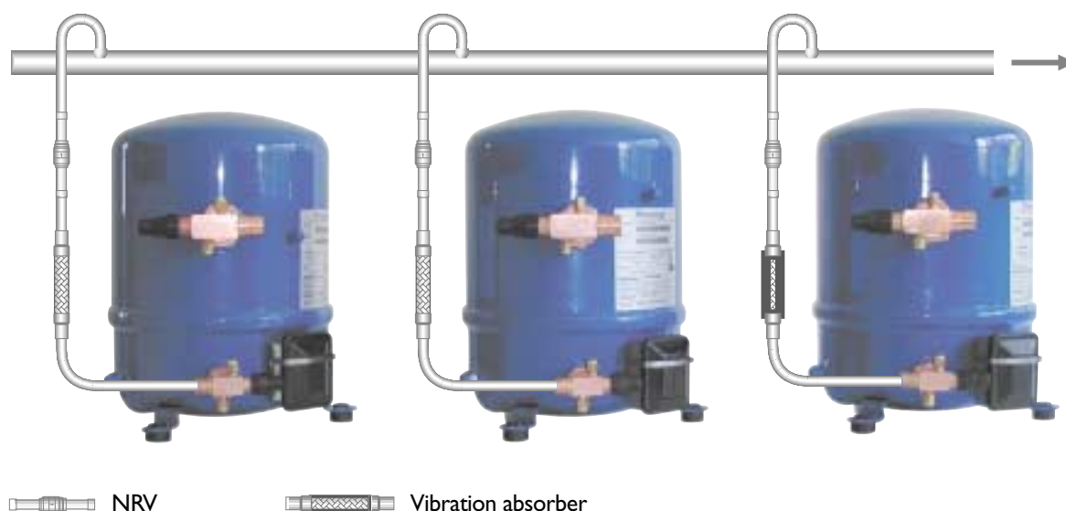
Figure 3.7 Discharge header above compressor discharge connections.
