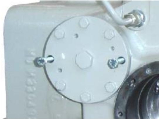
Put two long bolts in place
