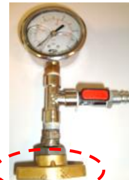
Pressure supply plug with Mano
