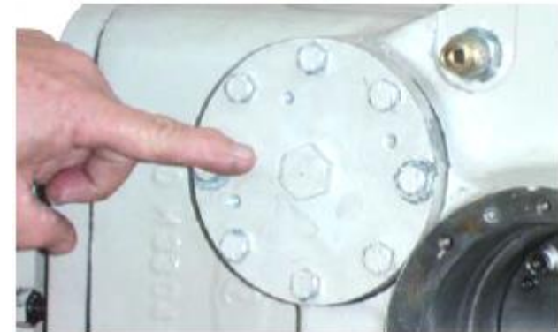
Re assemble without spring
