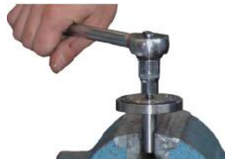
In order to separate spindle / plate, soft jaws can be used
