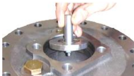
Remove spindle/plate
