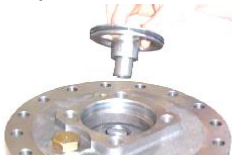
Remove the valve support
