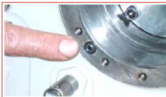
Oil line to unload valve
