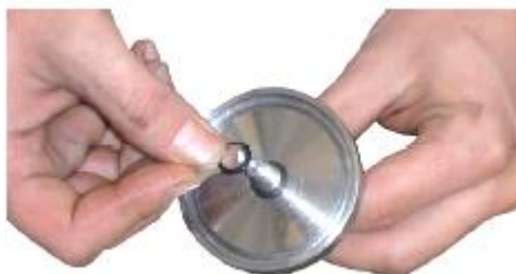
Replace O-ring on spindle
