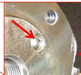
Ball inserts on cylinder cover
