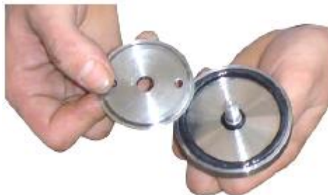
Remove plate retainer
