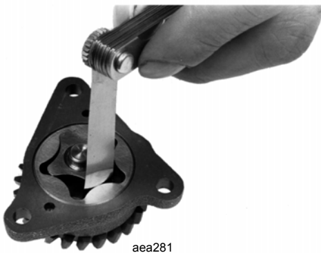
Checking Clearance Between Inner Rotor and Outer Rotor
