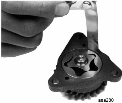
Checking Clearance Between Oil Pump Body and Outer Rotor
