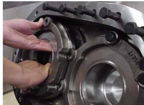
Fig. 5-19 Removal of the Valve Plate
