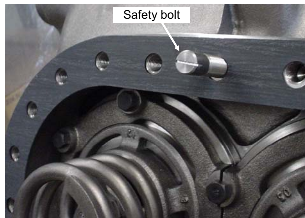
Fig. 5-8 Removal of Head Cover
