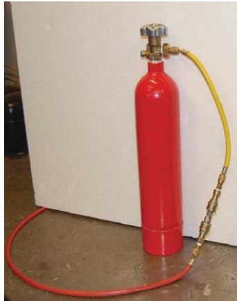
Vacuum suction of the filling hose
