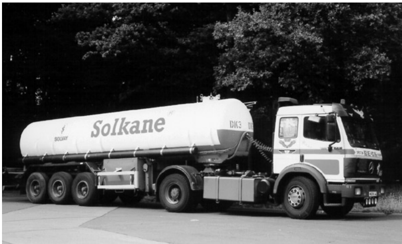
Road tanker with Solkane offer a capacity of approx. 20 t
