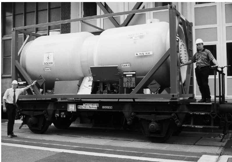
Tankcontainer filled with Solkane ready for Railtransport in front of Frankfurt plant
